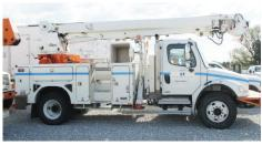
(56/67-742) 2004 Freightliner, model M2-160MD, 4x2, 62,628 miles, 6,942 hours, 5-speed manual transmission, Cat 3126 diesel engine, regular cab, with 2003 Altec D947TR digger, winch, a/c, cruise control, no power options, remotes do not work Truck:1FVACYAKX4HM67710 MH:1003BA3871
