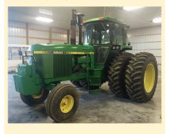
1978 John Deere 4640 Tractor, Quad Range, 10,031 hours, 20.8-38 Tires with 10 bolt Duals, Front wheel weights, triple hydraulics, 3 pt with quick hitch, Cab, Air, Radio, SN 4640H002675R
