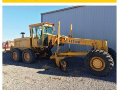
1989 John Deere 772BH Motor Grader, 4,665 hours showing, 14-24TC Tires, 5 shank rear scarifier, SN: 522743
