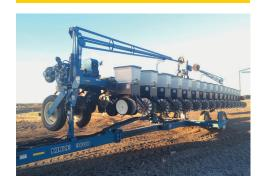
Kinze 3600 16R30" or 32R15" Planter, 2 pt. Hitch, Yetter Disk Openers w/ Finger Openers, ½ Have Notched Disk Openers only, Seed Firmers, Press Wheels, Corn & Bean Plates, Markers, AgLeader Monitor, Always Shedded, SN: 616583
